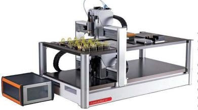
A two-level BSyS5.1/E (B-LAB) for automatic "organ-on-chip" cell culture with liquid and cell handling on the upper and a fluorescence microscope on the lower level
