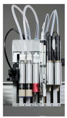
Example of a fully equipped pipetting head with (1) camera, (2+3) gripper/3-lumen pipette (one tool!), (4) FlipTube opener, (5) piezo tip + Z-sensor on one Z-axis, (6+7) nozzles for single-use needles and tips
