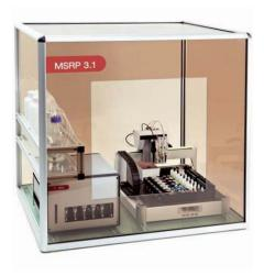
Small BSyS prototype with eight "kit plates" (containing septum vials, reactors, tubes, SPE columns etc.) and a needle holder, arranged as in a standard hot cell (W x D x H: 100 cm x 80 cm x 100 cm)
