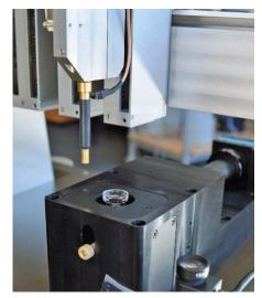
Micro-powder dispenser above a piezo-actuated powder reservoir. Two control cameras inspect the loading from the side and from below. Depending on the tip structure, different amounts ob beads can be transferred.
