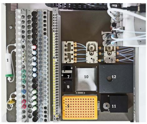
Typical objects on the work plate: (1) purification column; (2) sterile filter; (3) racks for tube adapters, closed/open crimp vials, reactor columns, septum vials, FlipTubes; (4) needle holder, (5) single-use pipette tips; (6) automatically replenished solvent reservoirs; (7) septum remover; (8) tip alignment station; (9) two wash stations for piezo tips; (10) piezo drying station; (11) stroboscope for piezo pipette check; (12) heated reactor chamber
