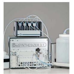
The F-Box, the electronic brain of the instrument and also central control station for pressure, vacuum and liquids, plus bottles with liquid level control and four syringe pumps for dispensers
