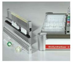
Racks removed from the robotic unit and replaced with holders for microtitre plates. Holders for slides exist, too.
