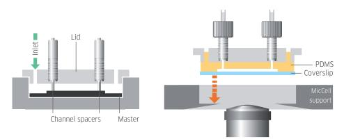
Moulding of the PDMS channel plate in the casting station (left) and mounting it in an inverted microscope (right). PDMS can be replaced by other materials, e.g. foils.
