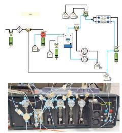
Detail of the GeSiM Fluidics software (example) and corresponding F-Box with selector values, syringe pumps and Peltier cooler with temperature control
