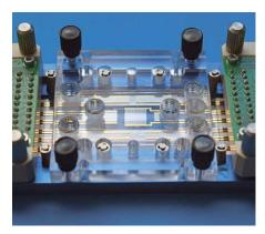
MicCell with microelectrodes structured on a 25x75 coverslip and connected via spring-loaded contacts
