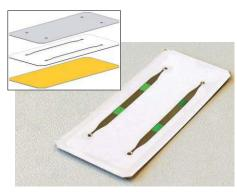
Biosensor cell made of three foils: transparent cover foil with holes, white channel foil, PC foil with four sensor pads (nanoimprinted in a GeSiM µCP4.1 and gold-coated). Used in a MicCell with near-infrared LEDs and wavelength-dependent photodiodes.
