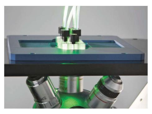
The MicCell is set up by casting a polymer channel plate, adding a coverslip, mounting it in the support and doing experiments under microscope control. The MicCell is ideal for rapid prototyping; making a new channel requires only a new silicon master that you can order from GeSiM.
